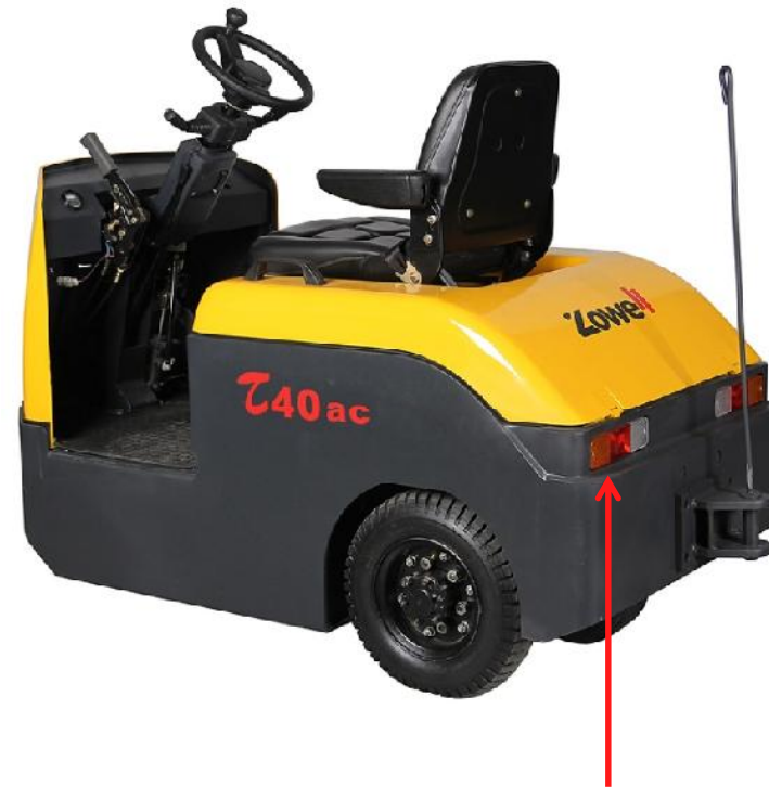
Tricolor taillight for braking, turning, backward
